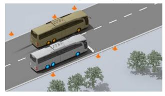
By constantly comparing the data, the electronic braking assist system immediately detects if the speed at which the brake pedal is pressed suddenly exceeds the usual level, and in such situations automatically boosts the maximum braking power to within fractions of a second. This significantly shortens the stopping distance of the vehicle.
