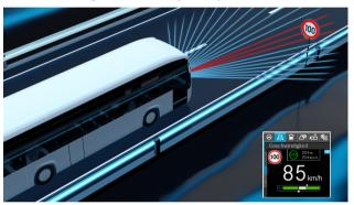
The innovative Traffic Sign Assist offers maximum safety and comfort on the road. Thanks to GPS and camera support, the vehicle speed is constantly compared with the current traffic regulations.
