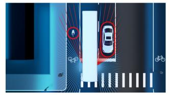
Sideguard Assist 2 is a safety assistance system that supports the driver in critical situations when turning right or turning left when visibility is possibly restricted. The system is designed to help detect moving obstacles within the system limits, and warns the driver so as to avoid critical situations or reduce the consequences of accidents when turning off or changing lanes.
