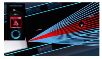
The emergency braking system ABA 6 assists the driver by automatically initiating emergency braking if there is a risk of rear-impact collision with vehicles in front or stationary obstacles. It also detects moving or stationary persons and cyclists in front of the vehicle. The system reacts to this with an acoustic and visual warning to the driver as well as an automatically initiated partial braking or emergency braking.
