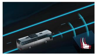
Lane Assist (SPA) detects when the vehicle unintentionally leaves a marked lane. If it crosses the markings, the driver is warned by a clear vibration through the driver's seat.
