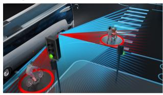
Sideguard Assist is a safety assistance system that supports the driver in critical cornering situations where visibility on the right side (curb side) may be limited. When turning or changing lanes, the system is designed to help avoid critical situations within the system boundaries or reduce the consequences of accidents.
