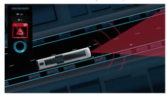
ABA 5 supports the driver in an imminent collision with stationary objects, moving objects and moving pedestrians. If a collision is imminent, the ABA 5 can carry out automatic emergency braking within the system limits. The system can thus reduce or, in ideal conditions, completely prevent accidents.
