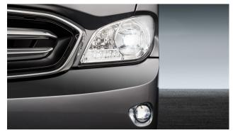
The high beam assistant automatically switches the high beams on or off depending on traffic, so that optimum illumination of the road is always ensured. When active, the system contributes to greater safety through improved lighting conditions and optimized illumination, and increases driving comfort and safety.
